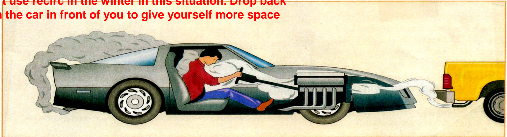
In heavy traffic, your intakes might draw in carbon monoxide from the exhaust of the car ahead.
