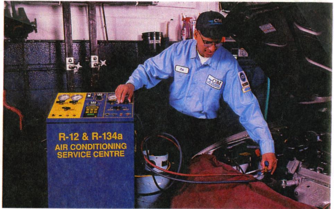
Refrigerant recovery systems are used on older vehicles to keep CFCs from escaping into the atmosphere.
